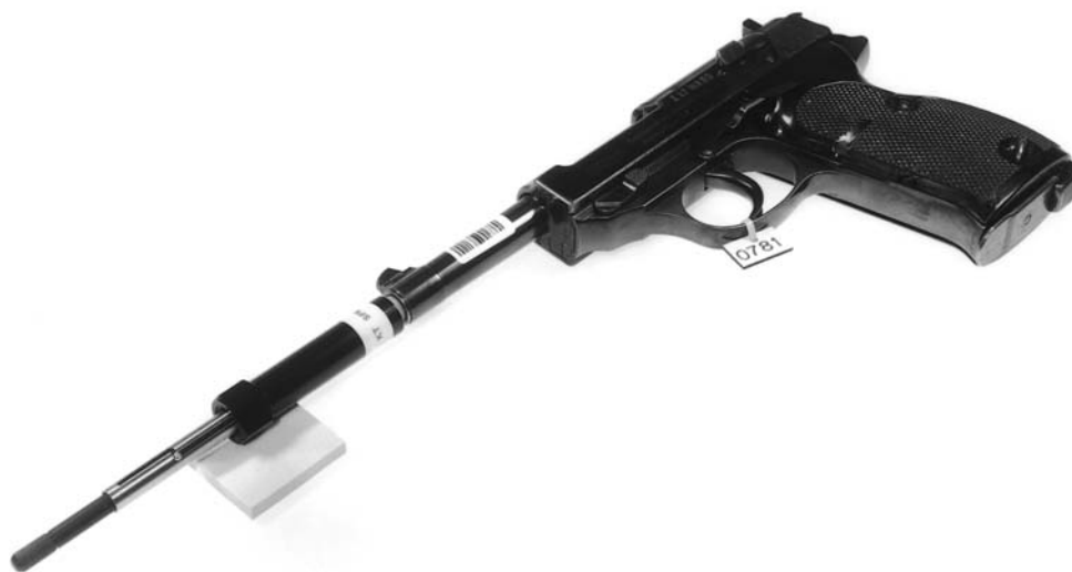
FIG. 1—Sampling from pistol barrels. The SPME fiber is exposed to the atmosphere inside the barrel for 40 min at room temperature. The pistol shown is a Walther of 7.65 mm caliber. Note the use of a cork in the pistol muzzle. The needle of the SPME device is pushed inside the barrel through the small aperture in the middle of the cork. The sampling position and geometry is thus kept constant.
